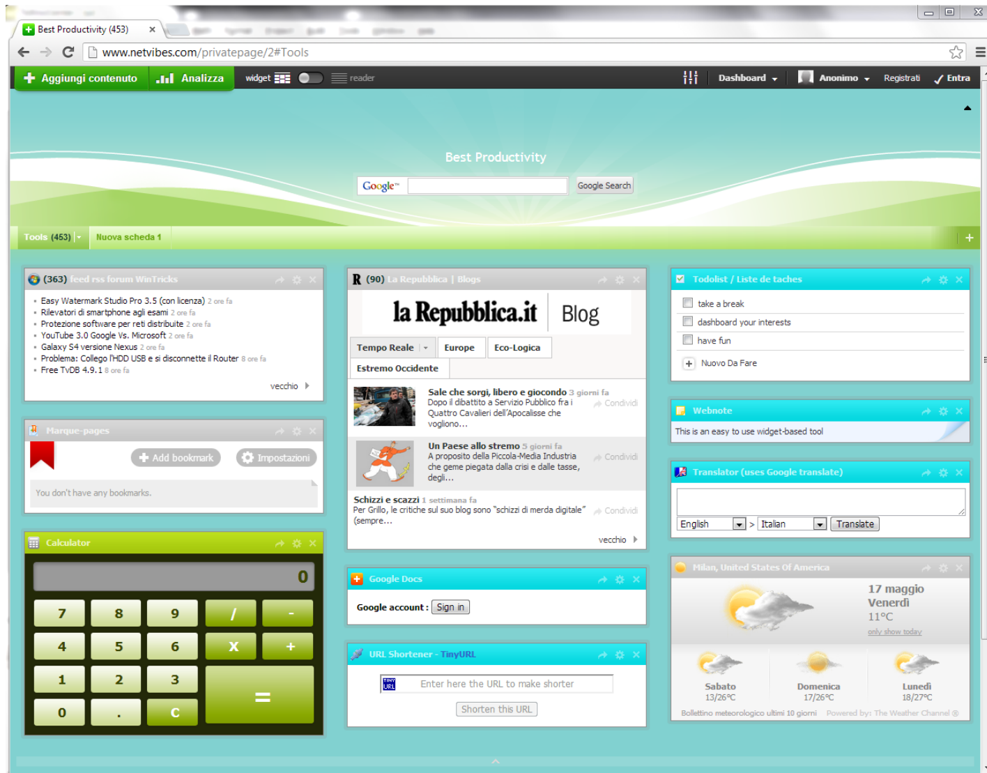
Fig. 6.14 An example of widget-based mashup created using the Netvibes platform. Different areas of the page correspond to different viewports, each one displaying the content of a different widget.
