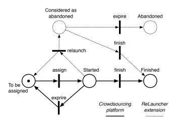
Figure 2. Petri Net modeling the execution semantics of assignments when executed with ReLauncher (dashed) integrated into a crowdsourcing platform (solid). Tokens correspond to assignments to be processed by workers.
