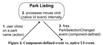
Essentially, user actions trigger both native UI events and component-defined events. However, native UI events are captured by the underlying UI toolkit and processed by the components internally, whereas component-defined events (which signal state changes) are exposed externally. It is up to the component to define and implement the relationship between native UI events and component events that signal state changes.
